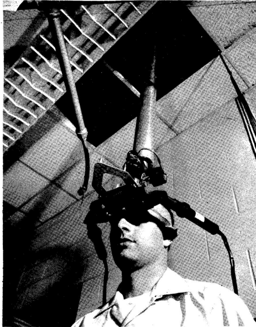
FIGURE 4—The ultrasonic head position sensor in use
